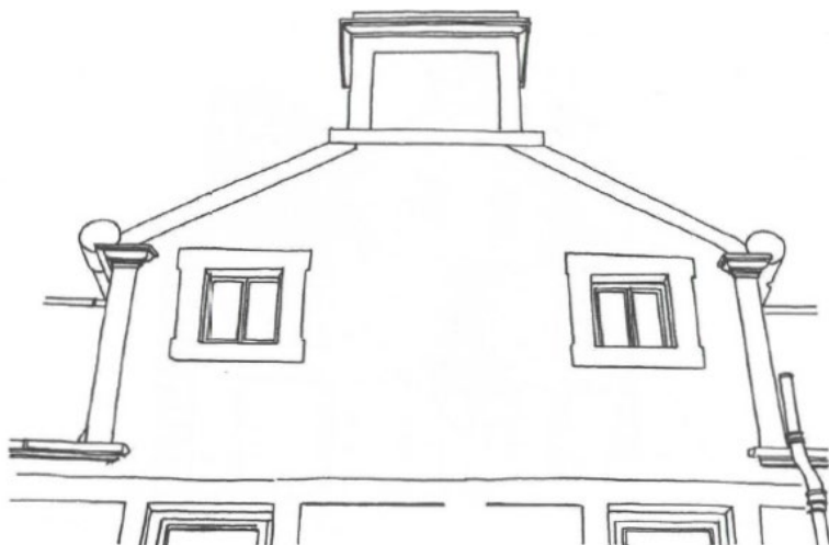
22. The nepus gable of The Smugglers Tavern, High Street, Beith, a late 18th building. Note the rolled skewputs.
