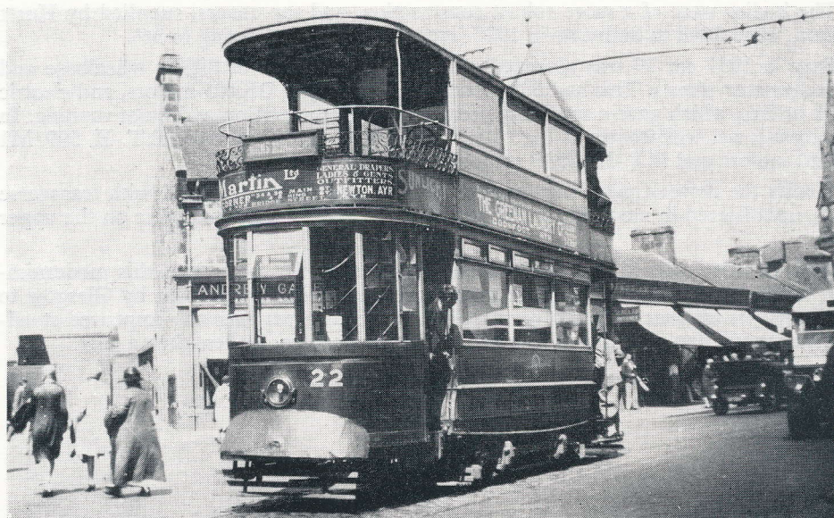
Car 22 at Prestwick in 1929 after addition of top cover and vestibuled platforms. The driver is looking out through the front exit.
